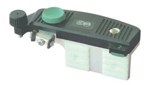
The top tool for re-setting or stripping the plastic sidewalls on skis or snowboards. Especially works to to strip away the second edge and sidewall on capped race skis. Replaceable tungsten carbide blades provide 2 round radius and square shapes. This tool provides precise adjustment of cutting depth on all axis.
